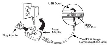
Option 2: Charging from a high-power USB port on a host device
