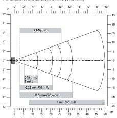
\* The reading distances given are typical reading distances measured in an office environment (200 lux)
