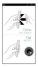
The cloning feature allows the settings of a device to be wirelessly cloned to another device within range.
