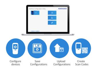
DXU can configure a wide variety of device parameters, including the scanner and most decoding parameters, the touch screen and the keyboard, interfaces such as NFC, Wi-Fi, Bluetooth, USB, and Ethernet, device settings such as date, time, time zone, and power management, and security settings such as password access. DXU can also configure communication parameters between the application that runs on a PC and the client applications that run on the device.
