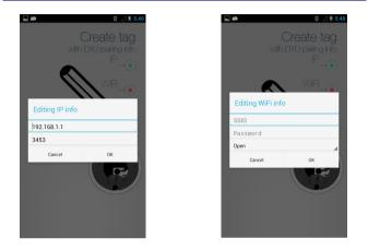
When the tool is launched from the device, the DXU Desktop IP and port information must be entered by the user. The Wi-Fi SSID, password and security type are automatically set to the actual Wi-Fi connection, unless the device is not connected to any network or there is any problem in fetching such information.
