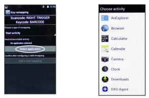
Select the desired application and then tap **Add a new mapping**. A window displays showing the new keymap:
