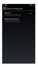
By default, the DL-Axist is configured to obtain IP addresses automatically via DHCP server. Alternatively, the device can be configured to use a statically assigned IP address.
