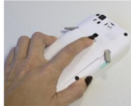
3. Rotate the latches to the lock position to lock the cover:
