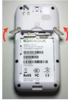
2. Insert the battery pack into the slot, bottom first, and press it into place:
