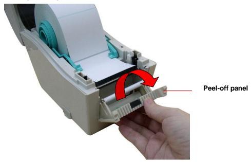
3. Lead the media through the backing paper opening, beneath the peel-off roller.
