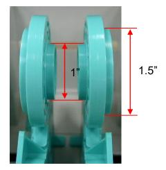
3. Separate the media holders to the label roll width.
