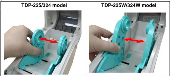
4. Place the roll between the holders and close them onto the core.
