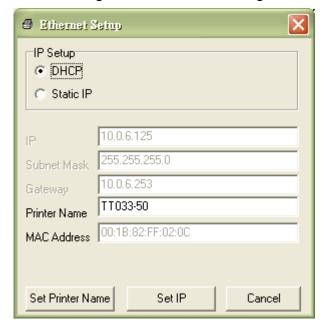
The default IP address is obtained by DHCP. To change the setting to static IP address, click "Static IP" radio button then enter the IP address, subnet mask and gateway. Click
