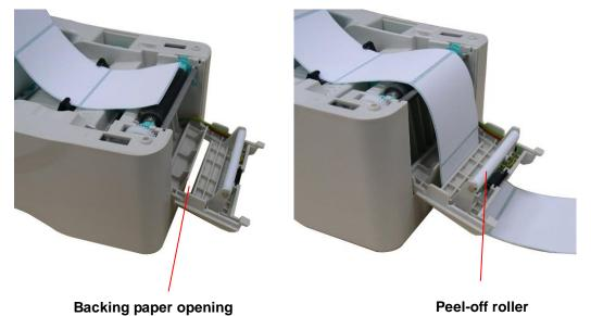
4. Push the peel-off panel back to the printer.
