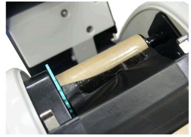
7. Turn the ribbon rewind gear until the ribbon plastic leader is thoroughly wound and the black section of the ribbon covers the print head. Close the ribbon access cover and the top cover.
