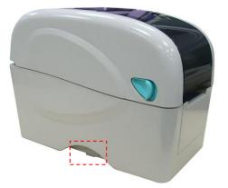
2. Insert the MicroSD card into the socket.
