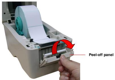
3. Lead the media through the backing paper opening, beneath the peel-off roller.
