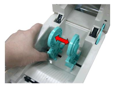
4. Place the roll between the holders and close them onto the core. Place the paper, printing side face up, through the media guides, media sensor and place the label leading edge onto the platen roller.
