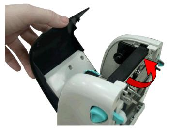
4. Insert the paper core right side onto the rewind hub. Align the notches on the left side and mount onto the spokes.
