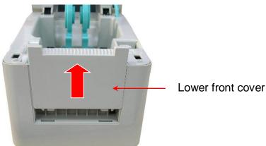
3. Disengage the platen holder tabs from the lower inner cover by pulling out the right side and left side tabs. Alter the both side tabs into the 90 degree position for thick label.
