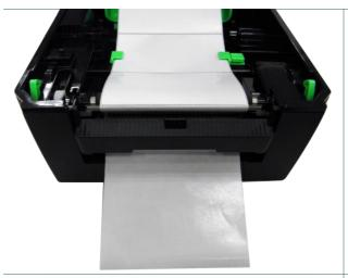
6. Close the peel-off cover and printer cover. Printer is ready for peel-off mode.
