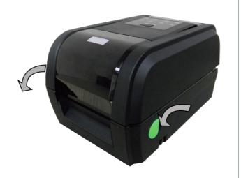
1. Open the printer top cover by pulling the tabs located on each side towards the front of the printer then lift the top cover to the maximum open angle.
