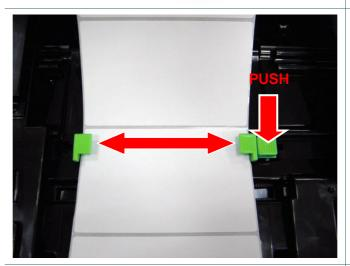
5. Move the media guides to fit the label width by pushing the media guide adjustment button.
