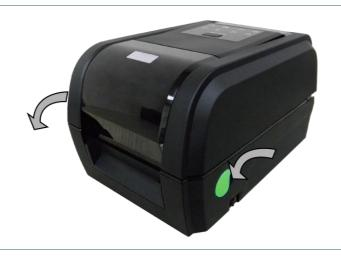
1. Open the printer's top cover by pulling the top cover open levers located on each side of the printer and lifting the top cover to the maximum open angle.
