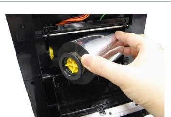
Note: The yellow part of spindle is in left side. 6. Install the ribbon right side onto the supply hub first then align the notches on the left side and mount onto the spokes.
