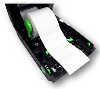
4. Place the paper, printing side face up, through the media sensor and place the label leading edge onto the platen roller.
