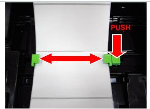
Move the media guides to fit the label width by pushing the media guide adjustment button.
