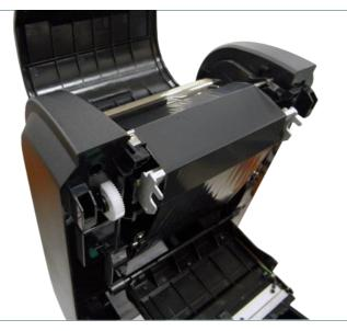
7. Stick the ribbon onto the ribbon rewind paper core.
