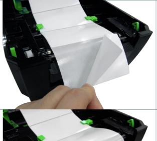
Open the peel-off cover. Feed the liner into peel-off cover slot.
