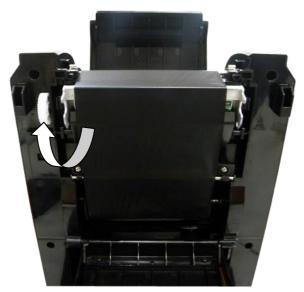
8. Turn the ribbon rewind gear until the ribbon plastic leader is thoroughly wound. Close the ribbon access cover and the top cover.
