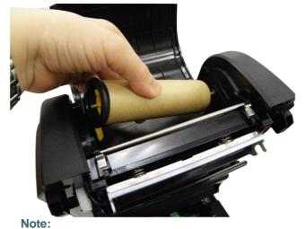
4. Install the paper core right side onto the rewind hub first then align the notches on the left side and mount onto the spokes.
