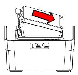
2. Insert the battery along the slot to the right side of charger station as pictured.
