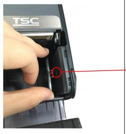
1. Open the printer top cover and install the media adapter in the media fixing hole as indicated.
