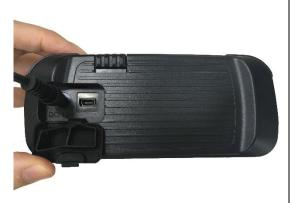
Open the interface cover and plug the power cord in to the power jack.
