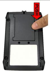
2. Push the right side of the battery clasp down and lock the battery.
