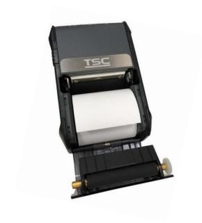
2. Place the media roll at the correct side, and pull out enough paper over the tear edge.
