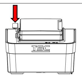
3. Push the battery clasp and properly install the battery, it will start charging.
