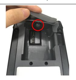
Remove the battery on the rear of the printer and lock the belt clip on the hole above the battery.
